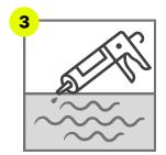
Apply Sika Dur 31 as a thinly spread layer or Hilti RE100 adhesive in this zigzags directly to surface. Make sure the full area for the mats is covered.
